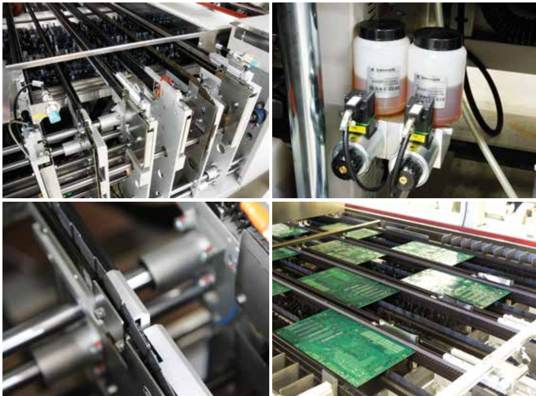
top left: dual lane transport, top right: chain oiler bottom left: lash chain centre board support, bottom right: quad lane transport
