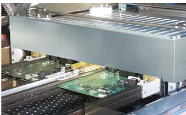
Opened vacuum chamber of the VisionXP+ Vac
